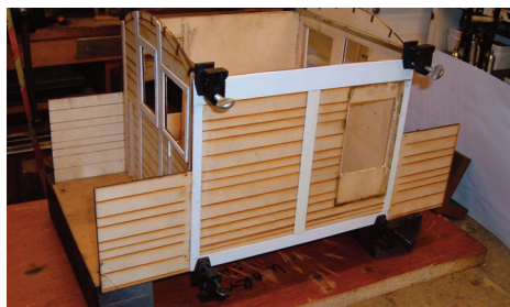
The body construction of Ivan's SR Brake Van
